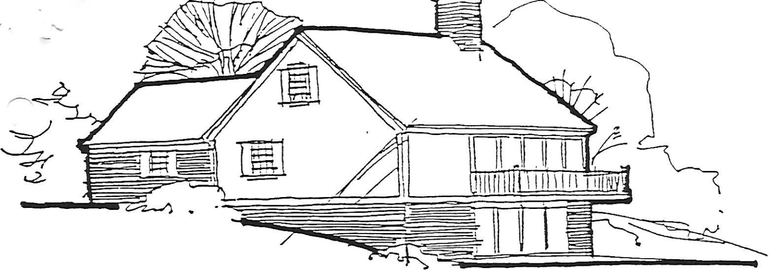
All Wood House with Masonry Wing, Chimney, and Foundation
