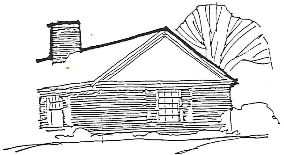
All Masonry Wing or House with Wood Gable
